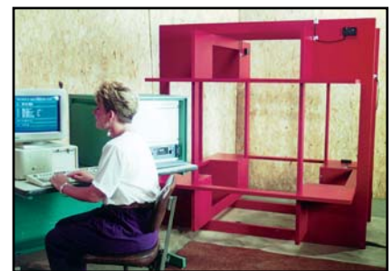
SQUARE, TRIAXIAL HELMHOLTZ SYSTEM Computer controlled, closed loop feedback system.
